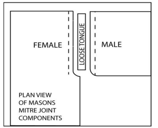
**Fig.13: plan view of the prepared joint showing the Loose Tongue**
