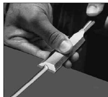
**Fig. 17 Removing glue deposits**
