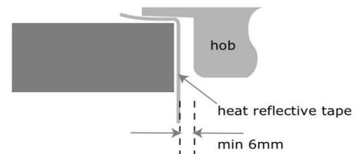
**Fig. 10 Application of Heat Reflective Tape**
