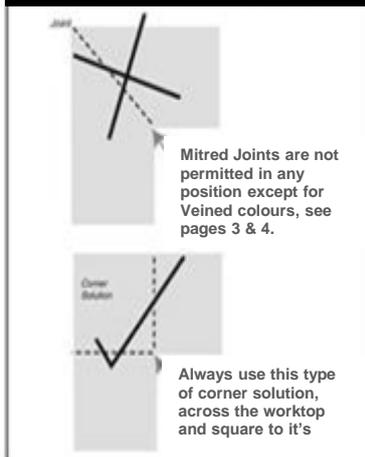
Where possible, for correct support, plan all joints to be situated directly above floor cabinet ends
