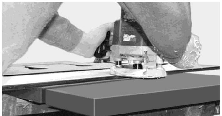
**Fig. 3: Cutting to size using a Router**
