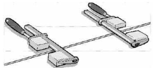
**Fig.15: Timber blocks and G-clamps**
