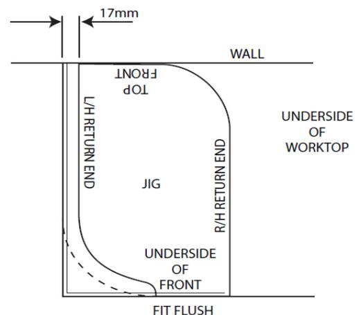
Fig.6: Positioning the Router Jig to remove the FSC Chipboard core, working from the underside of the Magna Worktop.
