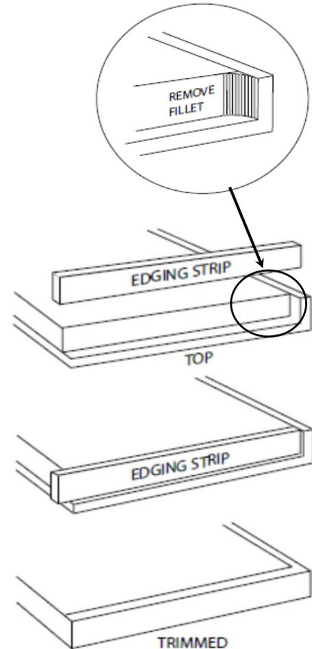
Fig. 4: Fitting the Edging Strip
