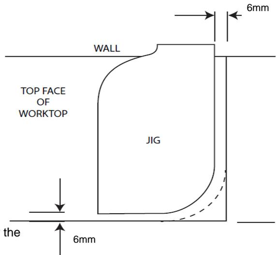
The method is to start at the step in the front edge of the jig and follow the full curve and along to the back edge of the worktop, removing the chipboard core into a curved shape set back from the front edge sufficiently to fit the 6mm thick curved edging strip.
