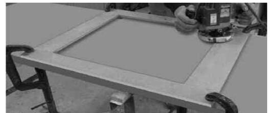
**Fig. 9 Hob/Sink template clamped in position**
